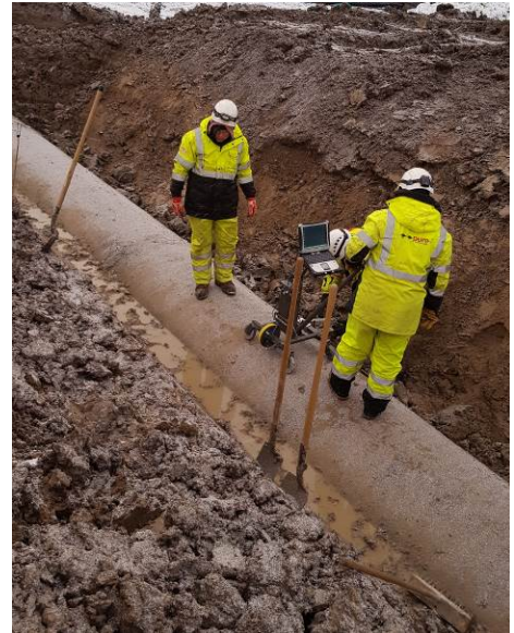
Figure 8b: Pure Technologies performs field confirmation of the distressed pipe location.
