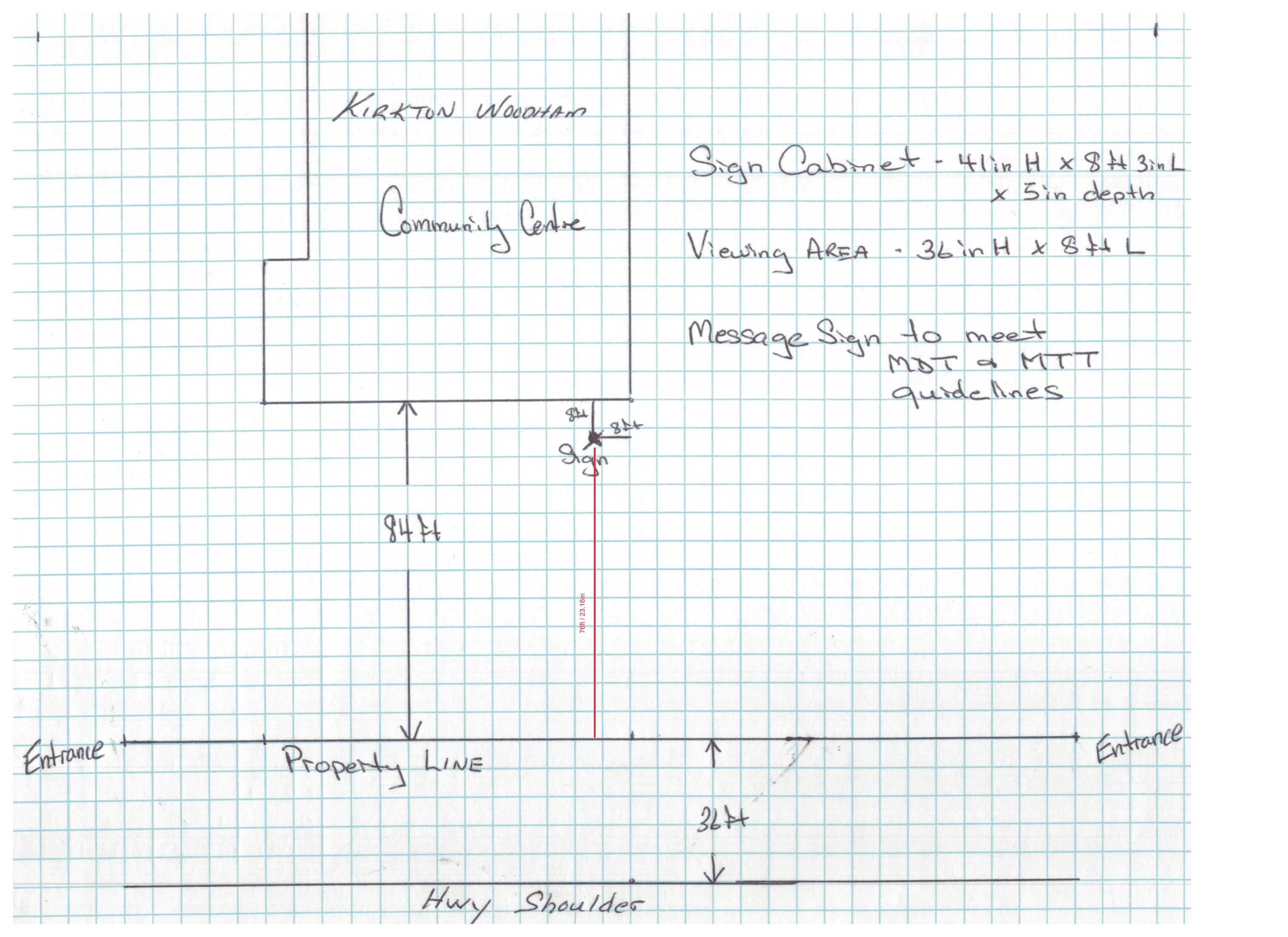
PROJECT: NEW Pylon Sign with white double high output LED Cabinet, and NEW Watchfire Video Displays.
